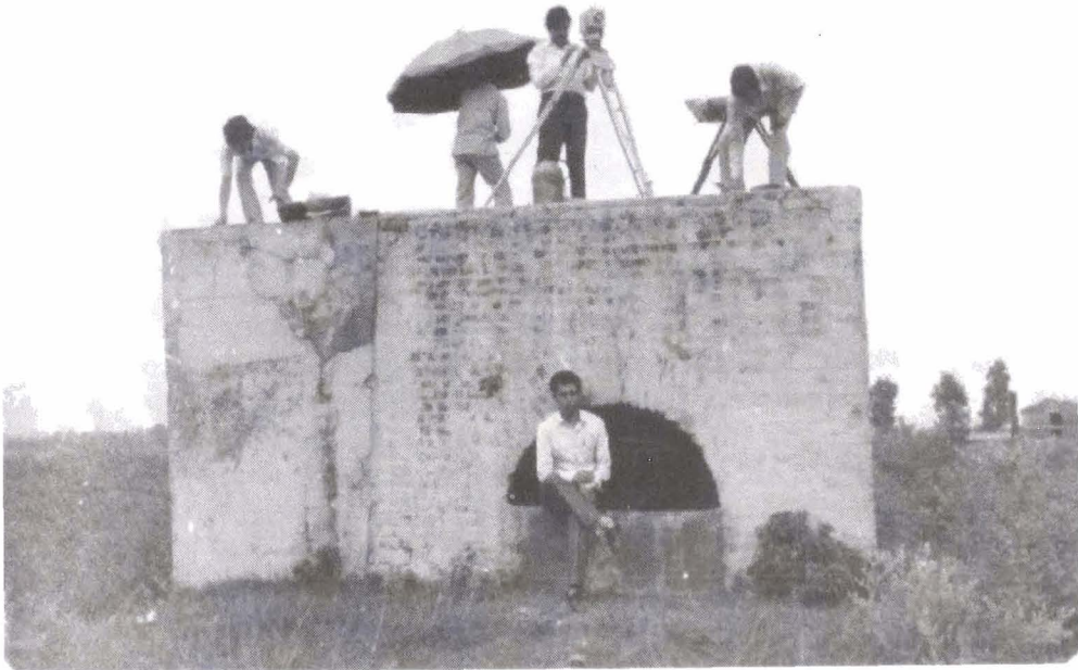
Figure 11 The west end terminal of the Dehra Dun baseline occupied by modern equipment.
